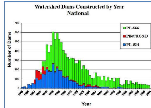
Many of the 11,845 flood control dams were built in the 1960s-70s and now are 50 to 60 plus years old. Most were designed for a 50-year service life.
